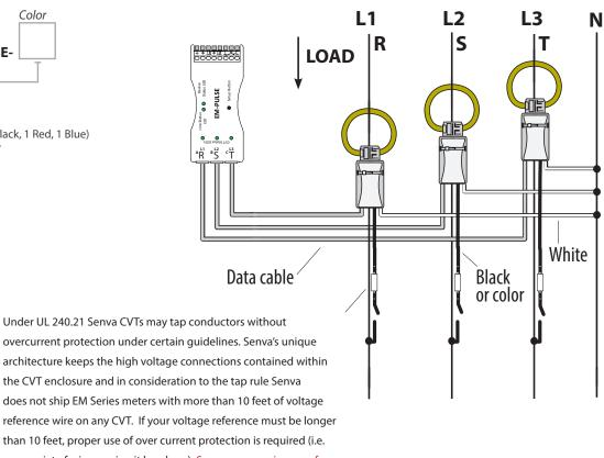
does not ship EM Series meters with more than 10 feet of voltage reference wire on any CVT. If your voltage reference must be longer than 10 feet, proper use of over current protection is required (i.e. appropriate fusing or circuit breakers.) See www.senvainc.com for additional information.
